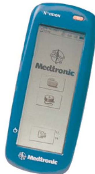
Fig. 11.5. Photograph of the Medtronic Synchronomed II hand-held programmer (picture courtesy of Medtronic)
